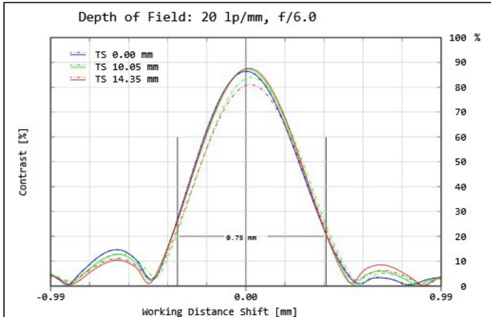
**Figure 4:** Polychromatic diffraction through-focus MTF at 20 linepairs/mm (image space). Contrast is plotted to two times the focus distance. Note object spatial frequency changes with working distance.
