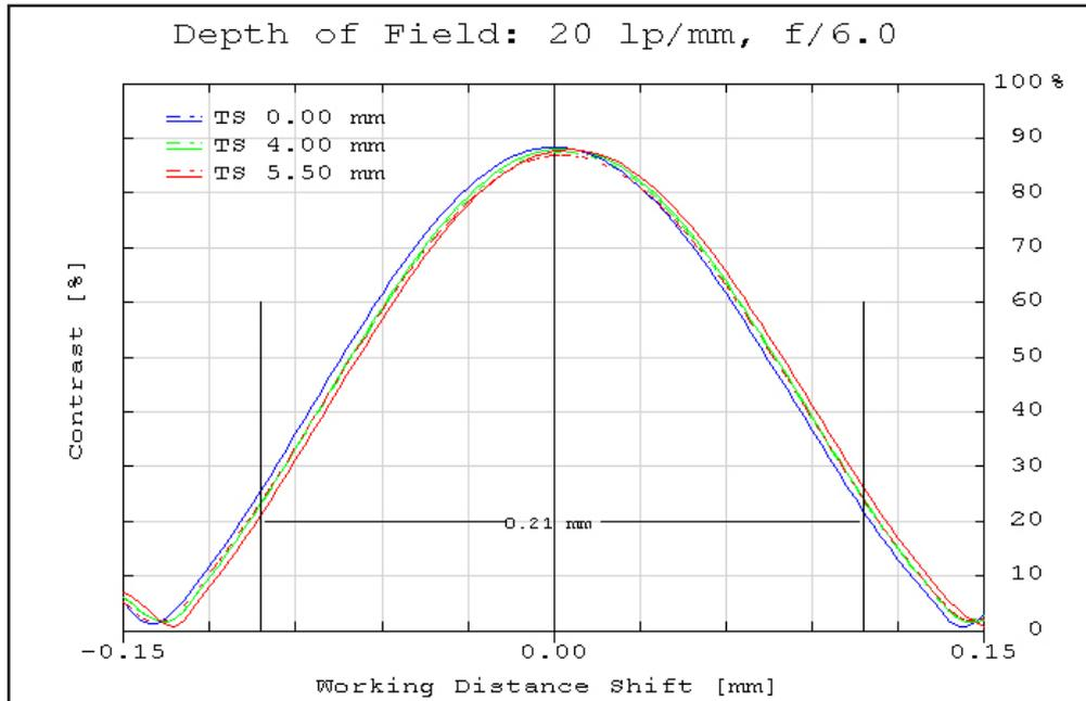
**Figure 4:** Polychromatic diffraction through-focus MTF at 20 linepairs/mm (image space). The depth of field at the maximum sensor format for the plotted frequency and  $f/\#$  at 20% contrast is indicated by the measurement bars.
