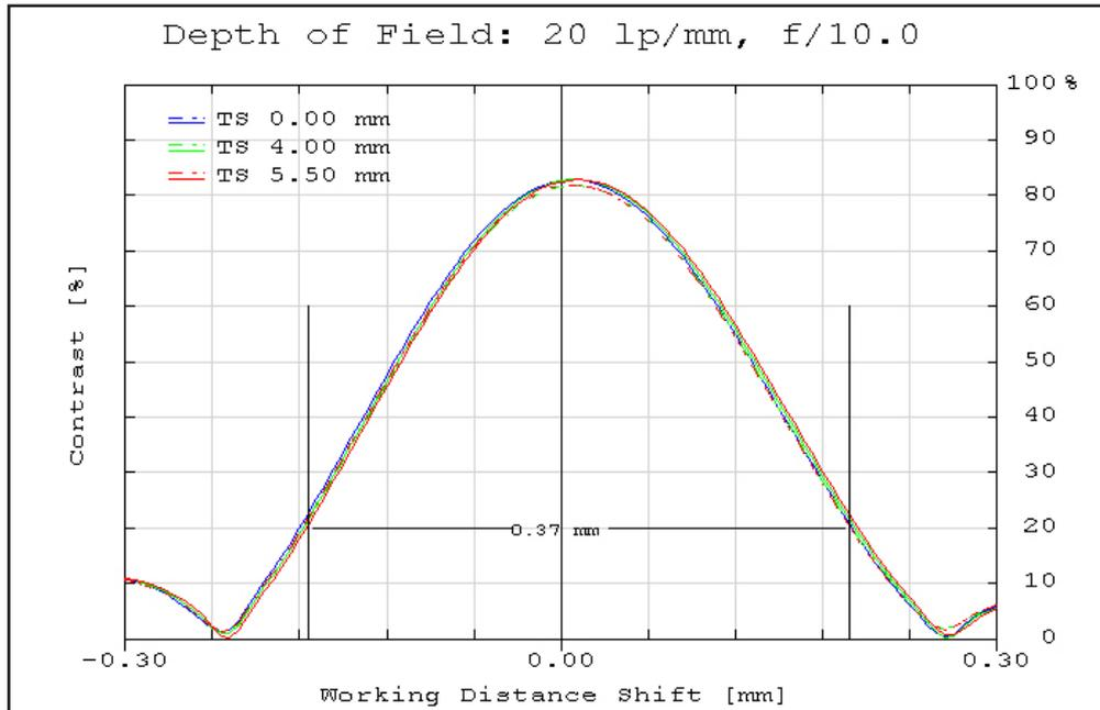
**Figure 6:** Polychromatic diffraction through-focus MTF at 20 linepairs/mm (image space). The depth of field at the maximum sensor format for the plotted frequency and  $f/\#$  at 20% contrast is indicated by the measurement bars.
