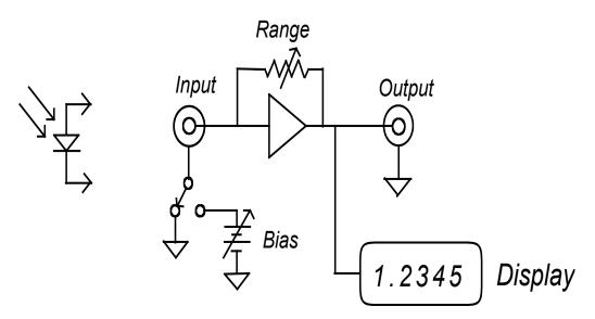
Current input to the unit generates a voltage across the range feedback resistor. This voltage is then measured and displayed in units of amperes. A variable bias voltage may be introduced in series with the detector in use. The output presented is calibrated such that 2.0000V represents the full scale range in use, e.g. 2.0000 V corresponds to 20.000 nA and so on.
