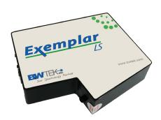
The Exemplar® LS is a smart CCD spectrometer optimized for low straylight by utilizing an unfolded Czerny-Turner spectrograph. It features on board data processing, USB 3.0 communication, and temperature compensation. The Exemplar LS is also optimized for multi-channel operation, featuring ultra-low trigger delay and gate jitter. Additionally, the Exemplar LS features a 2048 element detector and built-in 16-bit digitizer with greater than 2.0 MHz readout speed.
