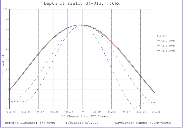
#34-013, 0.066X, 1" C-Mount TitanTL® Telecentric Lens, Depth of Field Plot, 377mm Working Distance, f11
