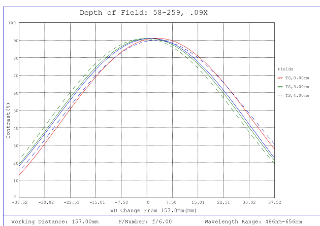
#58-259, 0.09X \frac{1}{2} " GoldTL™ Telecentric Lens, Depth of Field Plot, 157mm Working Distance, f6
