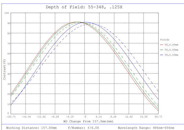
#55-348, 0.125X, 2/3" GoldTL™ Telecentric Lens, Depth of Field Plot, 157mm Working Distance, f6
