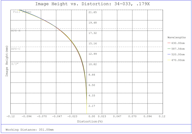
#34-033, 0.179X, 35mm F-Mount TitanTL® Telecentric Lens, Distortion Plot
