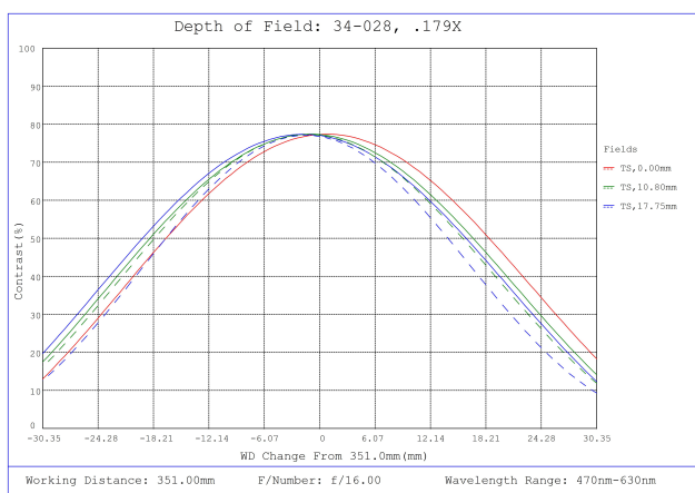
#34-028, 0.179X, 35mm M42 x 1.0 TitanTL® Telecentric Lens, Depth of Field Plot, 351mm Working Distance, f16
