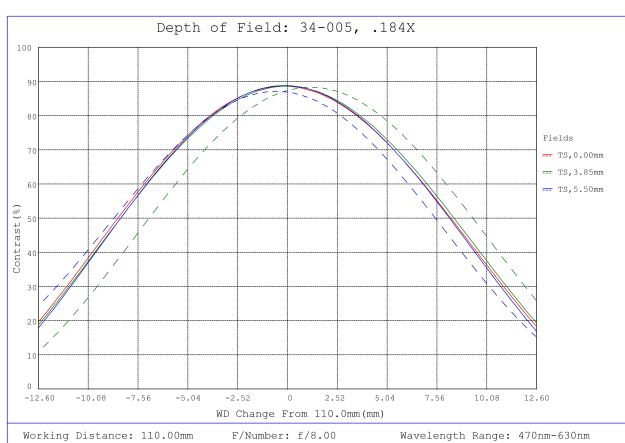
#34-005, 0.184X, 2/3" C-Mount TitanTL® Telecentric Lens, Depth of Field Plot, 110mm Working Distance, f8
