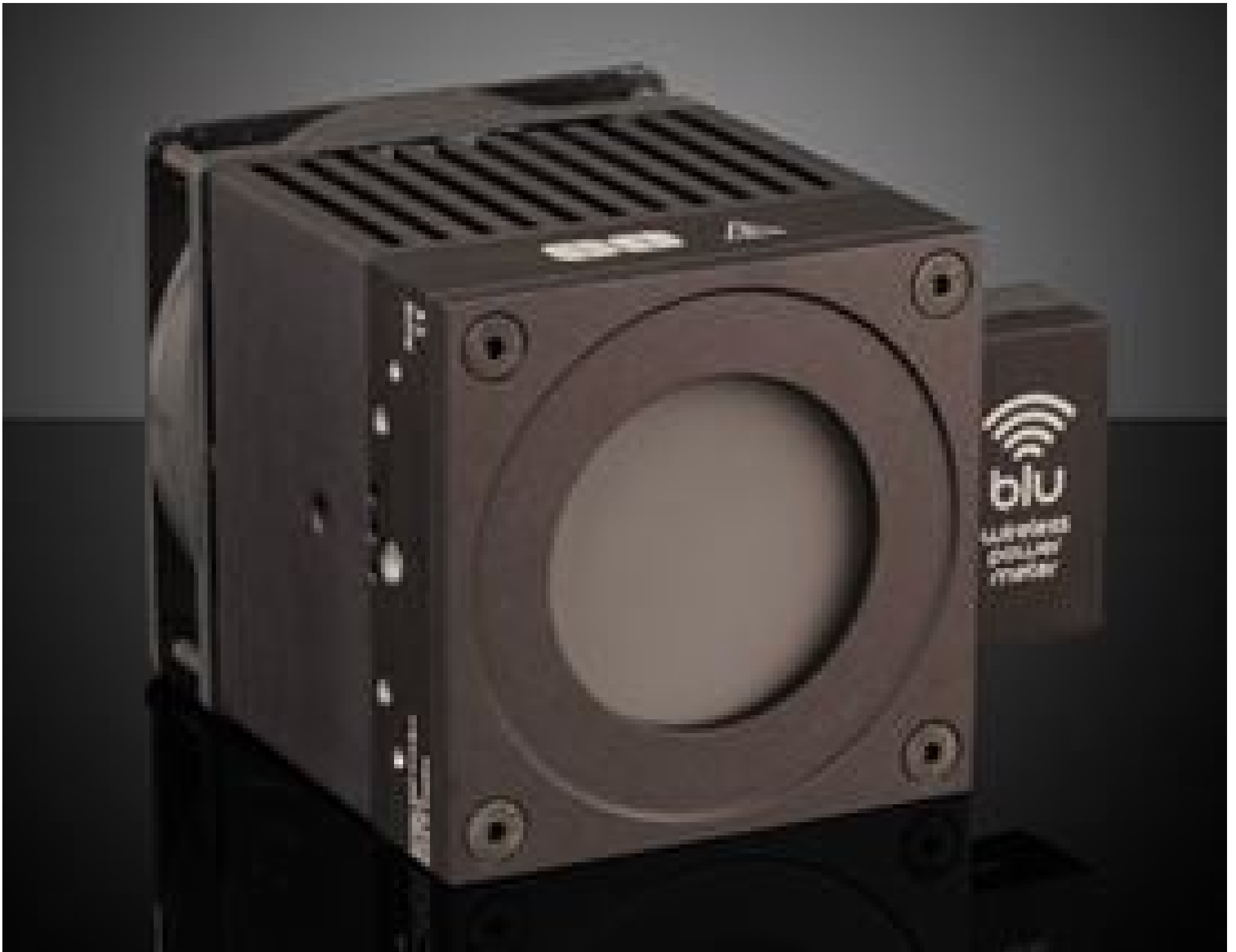
0.19 - 20 \mu\text{m} , 300W, Thermopile Wireless Power & Energy Detector
