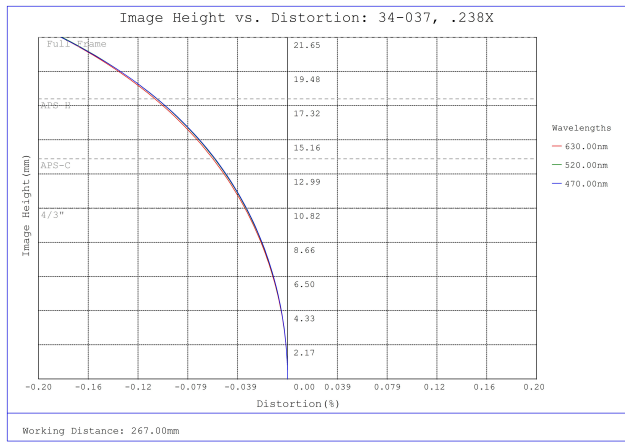
#34-037, 0.238X, 35mm M58 x 0.75 TitanTL® Telecentric Lens, Distortion Plot
