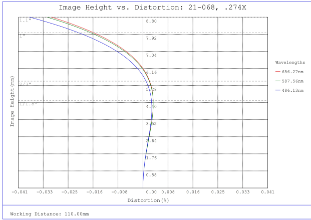
#21-068, 0.274X CobaltTL Telecentric Lens, Distortion Plot
