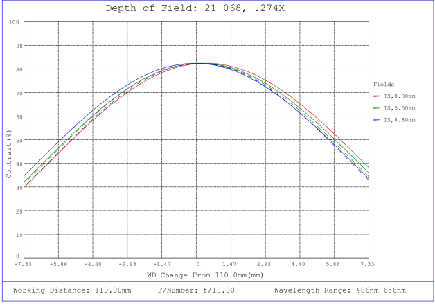
#21-068, 0.274X CobaltTL Telecentric Lens, Depth of Field Plot, 110mm Working Distance, f10
