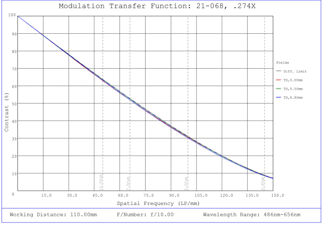
#21-068, 0.274X CobaltTL Telecentric Lens, Modulated Transfer Function (MTF) Plot, 110mm Working Distance, f10
