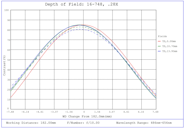
#16-748, 0.28X, 28.7mm TFL-Mount PlatinumTL™ Telecentric Lens, Depth of Field Plot, 182mm Working Distance, f10
