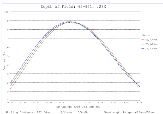
#62-921, 0.28X CobaltTL Telecentric Lens, Depth of Field Plot, 182mm Working Distance, f6
