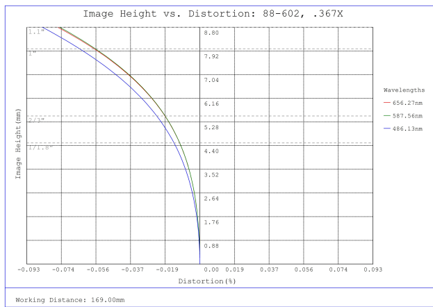
#88-602, 0.367X CobaltTL Telecentric Lens, Distortion Plot
