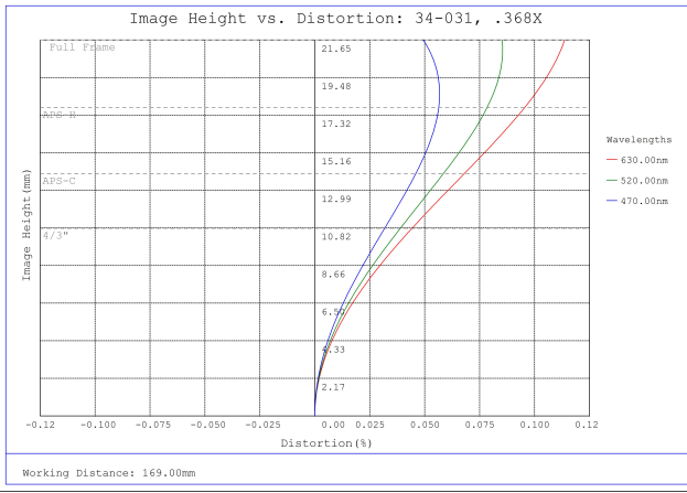
#34-031, 0.368X, 35mm F-Mount TitanTL® Telecentric Lens, Distortion Plot
