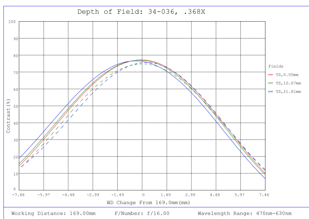
#34-036, 0.368X, 35mm M58 x 0.75 TitanTL® Telecentric Lens, Depth of Field Plot, 169mm Working Distance, f16
