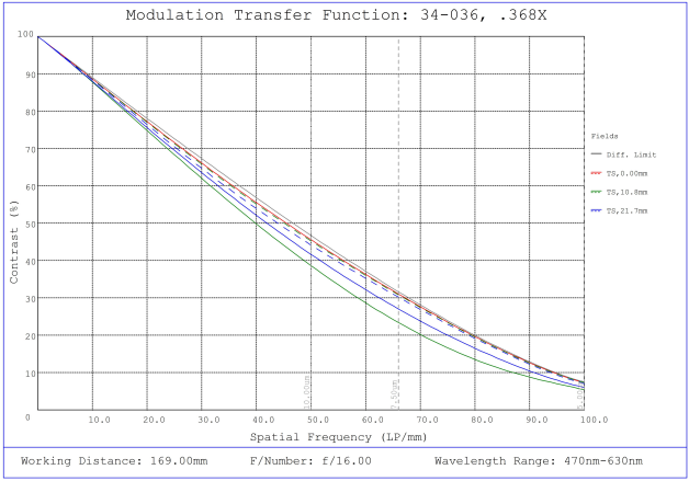
#34-036, 0.368X, 35mm M58 x 0.75 TitanTL® Telecentric Lens, Modulated Transfer Function (MTF) Plot, 169mm Working Distance, f16
