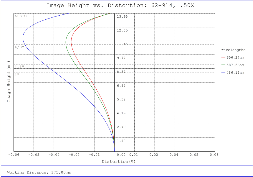
#62-914, 0.5X, 28.7mm M42 x 1.0 (19.53mm) PlatinumTL™ Telecentric Lens, Distortion Plot
