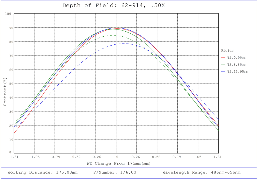
#62-914, 0.5X, 28.7mm M42 x 1.0 (19.53mm) PlatinumTL™ Telecentric Lens, Depth of Field Plot, 175mm Working Distance, f6
