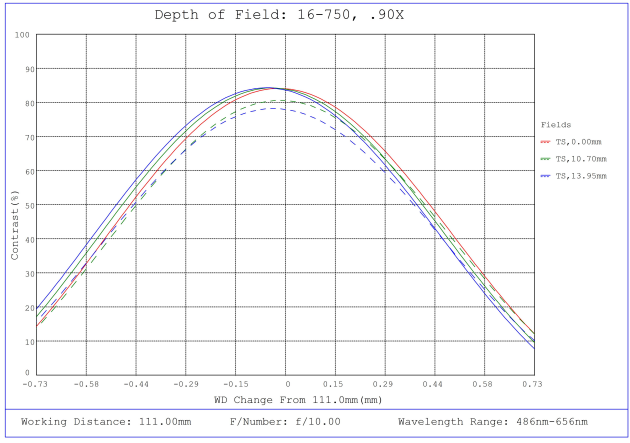
#16-750, 0.9X, 28.7mm TFL-Mount PlatinumTL™ Telecentric Lens, Depth of Field Plot, 111mm Working Distance, f10
