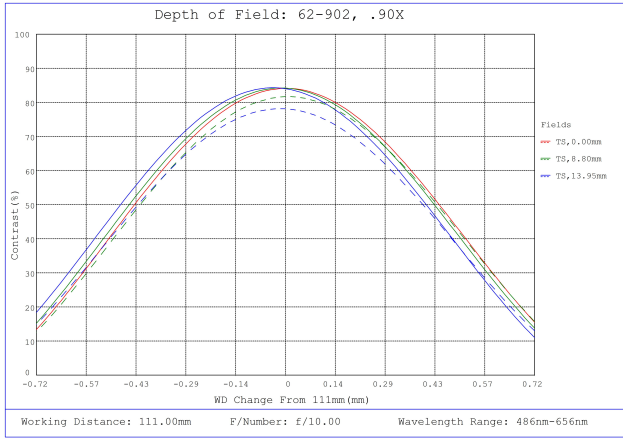
#62-902, 0.9X, 28.7mm F-Mount PlatinumTL™ Telecentric Lens, Depth of Field Plot, 111mm Working Distance, f10
