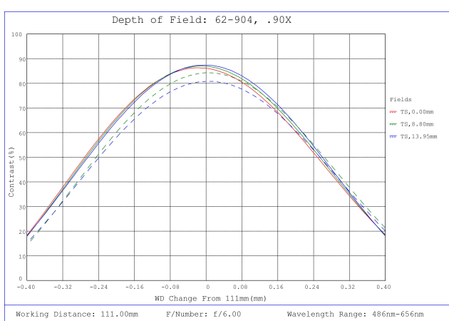
#62-904, 0.9X, 28.7mm M42 x 1.0 (19.53mm) PlatinumTL™ Telecentric Lens, Depth of Field Plot, 111mm Working Distance, f6
