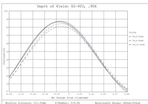
#62-903, 0.9X, 28.7mm M42 x 1.0 (6.56mm) PlatinumTL™ Telecentric Lens, Depth of Field Plot, 111mm Working Distance, f6
