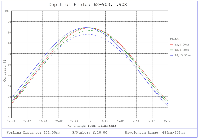
#62-903, 0.9X, 28.7mm M42 x 1.0 (6.56mm) PlatinumTL™ Telecentric Lens, Depth of Field Plot, 111mm Working Distance, f10
