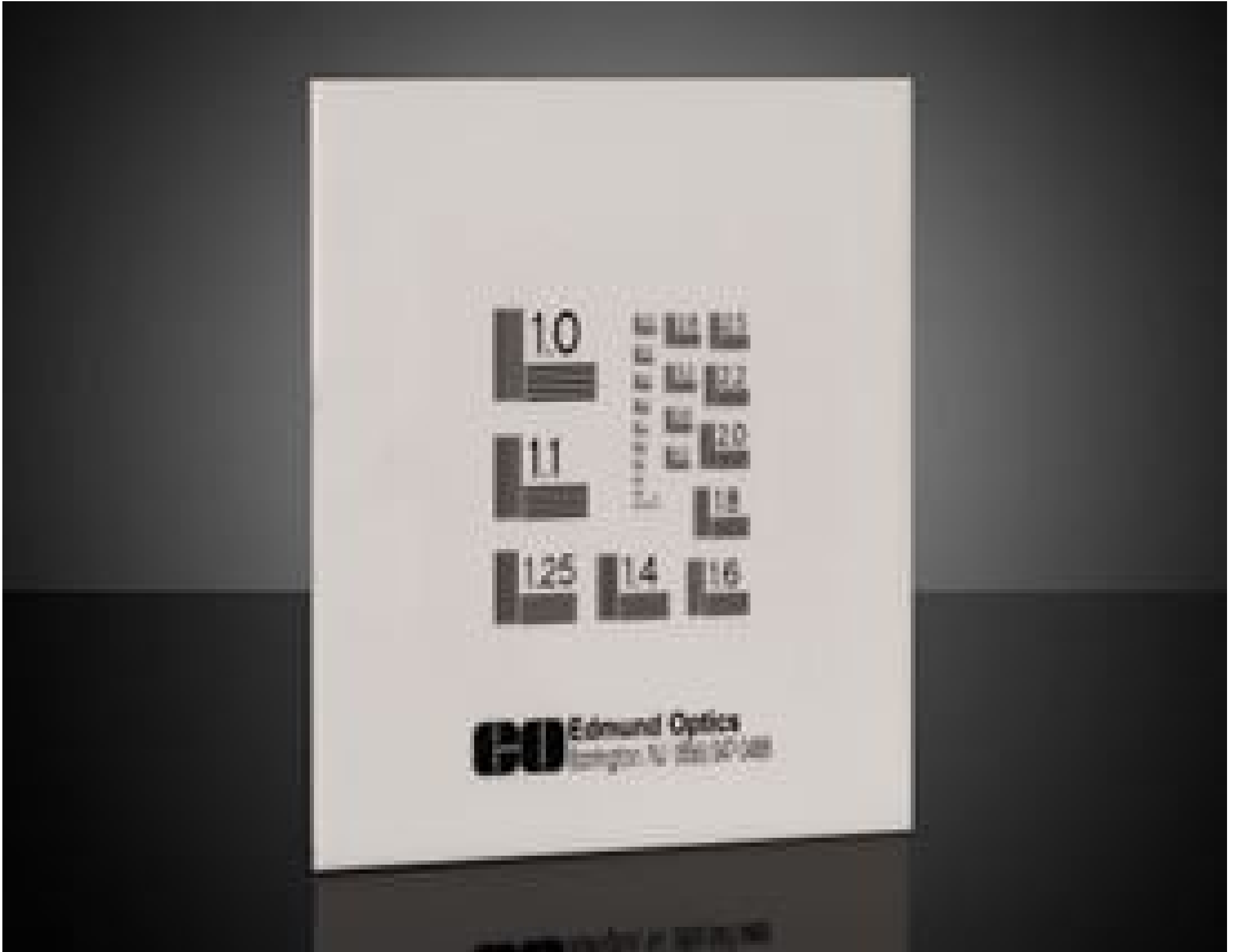
NBS 1963A Resolution Target
