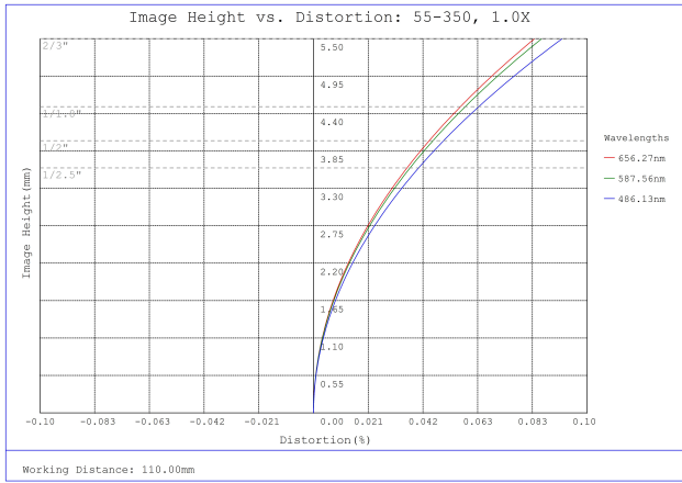
#55-350, 1.0X 2/3" GoldTL™ Telecentric Lens, Distortion Plot
