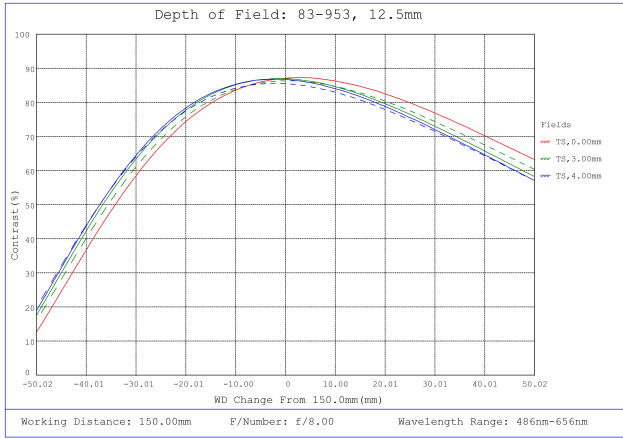
#83-953, 12.5mm FL f/8, Blue Series M12 Lens, Depth of Field Plot, 150mm Working Distance, f8
