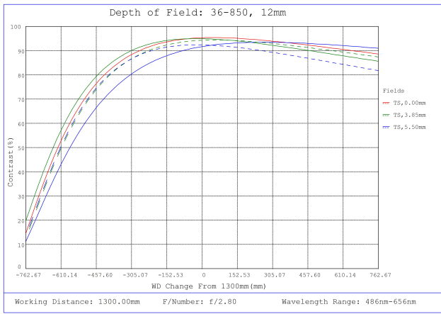
#36-850, 12mm f/2.8, 400-2000mm Primary WD, HRr Series Fixed Focal Length Lens, Depth of Field Plot, 1300mm Working Distance, f2.8
