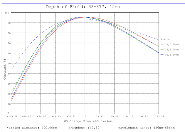
#33-877, 12mm, f/2.8 UCi Series Fixed Focal Length Lens, Depth of Field Plot, 400mm Working Distance, f2.8
