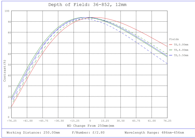
#36-852, 12mm f/4, 150-500mm Primary WD, HRr Series Fixed Focal Length Lens, Depth of Field Plot, 250mm Working Distance, f2.8
