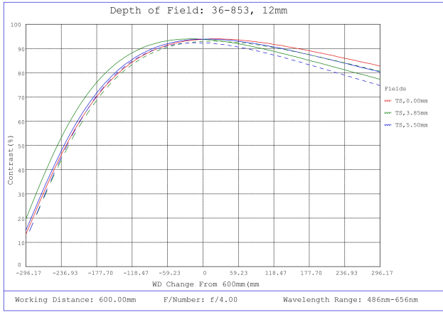
#36-853, 12mm f/4, 400-2000mm Primary WD, HRr Series Fixed Focal Length Lens, Depth of Field Plot, 600mm Working Distance, f4
