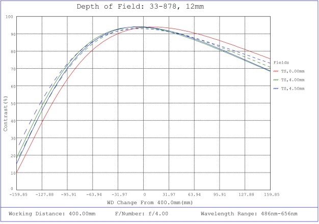
#33-878, 12mm, f/4 UCI Series Fixed Focal Length Lens, Depth of Field Plot, 400mm Working Distance, f4
