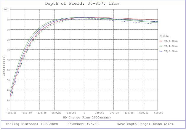
#36-857, 12mm f/5.6, 1000mm-∞ Primary WD, HRr Series Fixed Focal Length Lens, Depth of Field Plot, 1000mm Working Distance, f5.6
