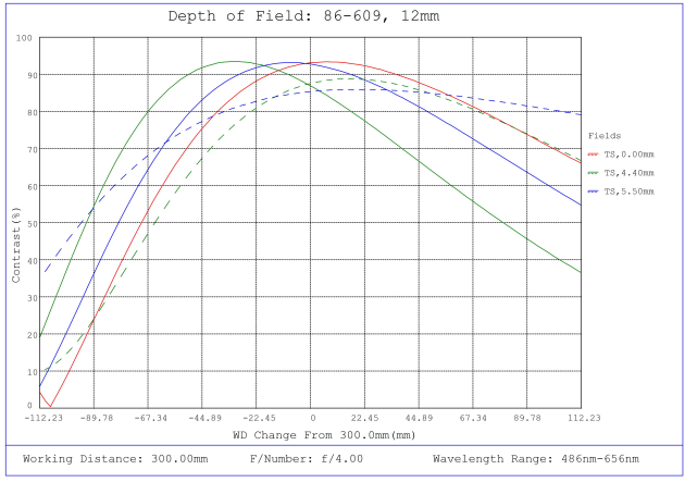
#86-609, 12mm, f/4 Ci Series Fixed Focal Length Lens, Depth of Field Plot, 300mm Working Distance, f4
