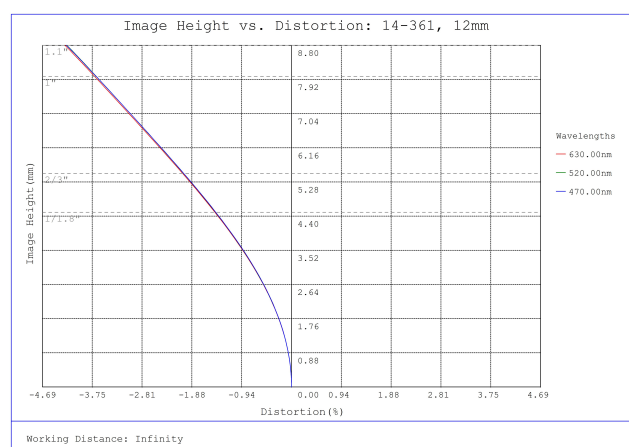
#14-361, 12mm LT Series Fixed Focal Length Lens, Distortion Plot
