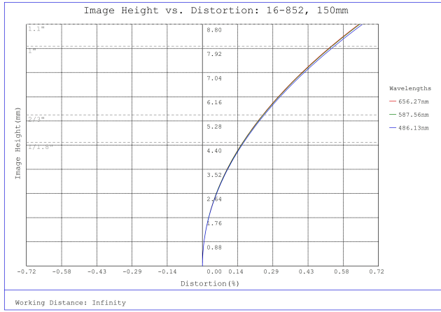
#16-852, 150mm, f/4 Athermal Lens, Distortion Plot
