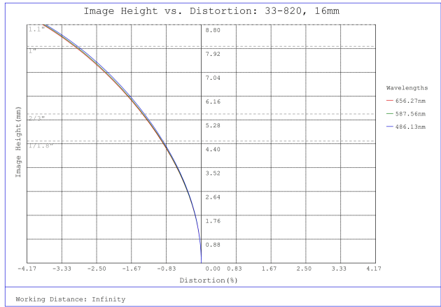
#33-820, 16mm f/16, HPi Series Fixed Focal Length Lens, Distortion Plot
