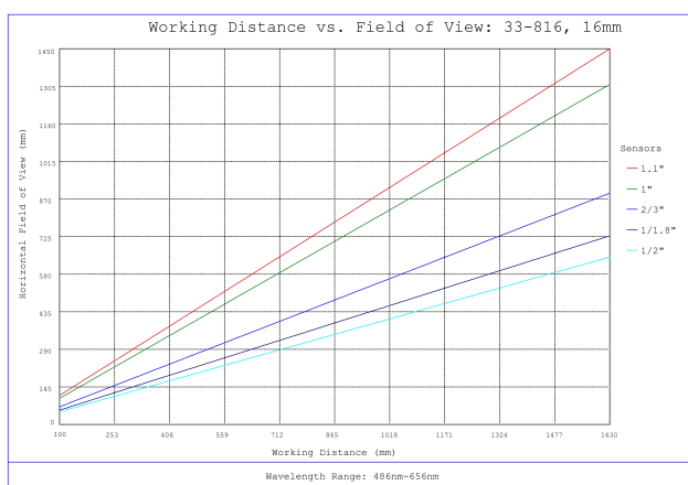
#33-816, 16mm f/4, HPI Series Fixed Focal Length Lens, Working Distance versus Field of View Plot
