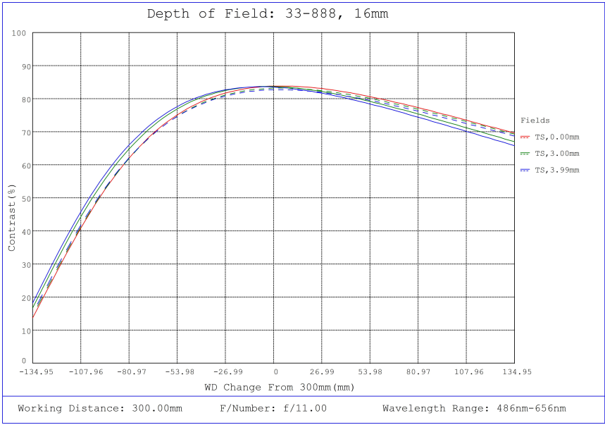
#33-888, 16mm, f/11 UCi Series Fixed Focal Length Lens, Depth of Field Plot, 300mm Working Distance, f11
