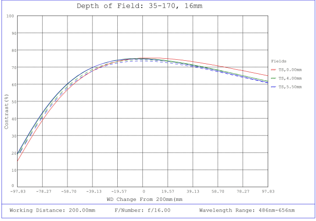
#35-170, 16mm, f/16 Cr Series Fixed Focal Length Lens, Depth of Field Plot, 200mm Working Distance, f16
