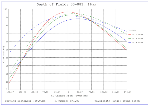
#33-883, 16mm, f/1.8 UCi Series Fixed Focal Length Lens, Depth of Field Plot, 750mm Working Distance, f1.8
