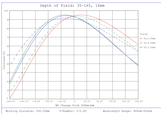
#35-165, 16mm, f/2.8 Cr Series Fixed Focal Length Lens, Depth of Field Plot, 500mm Working Distance, f2.8
