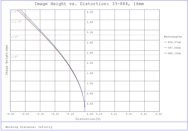
#33-884, 16mm, f/2.8 UCi Series Fixed Focal Length Lens, Distortion Plot
