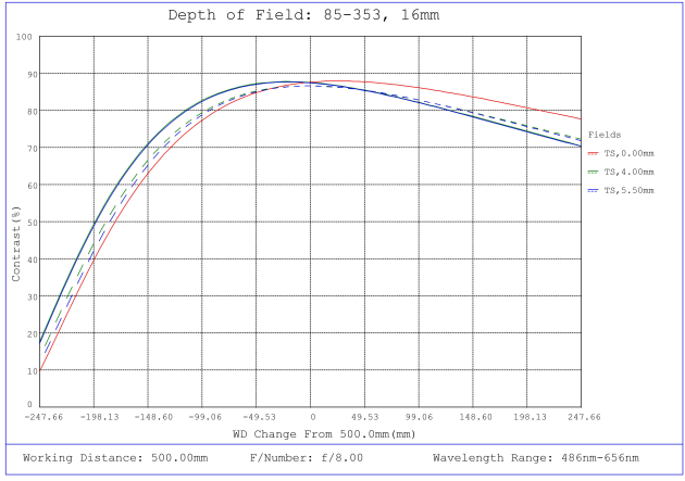
#85-353, 16mm, f/8 Ci Series Fixed Focal Length Lens, Depth of Field Plot, 500mm Working Distance, f8
