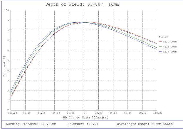
#33-887, 16mm, f/8 UCI Series Fixed Focal Length Lens, Depth of Field Plot, 300mm Working Distance, f8
