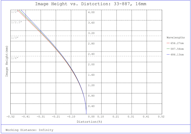
#33-887, 16mm, f/8 UCi Series Fixed Focal Length Lens, Distortion Plot
