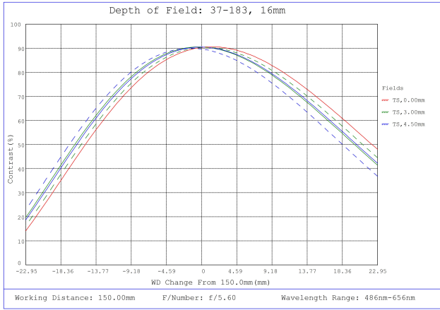
#37-183, 16mm FL f/5.6 Blue Series M12 Lens, Depth of Field Plot, 150mm Working Distance, f5.6
