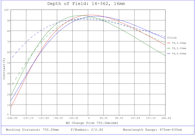
#14-362, 16mm LT Series Fixed Focal Length Lens, Depth of Field Plot, 750mm Working Distance, f2.8
